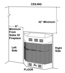
0" Minimum Clearance To Top Surface Of Carpeting, Tile Or Other Combustible Material
